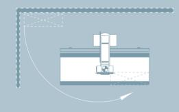
MULTIX Swing is specifically designed to provide a high degree of flexibility, even in a small room. The generator is integrated into the table and doe not require additional space. This integration also facilitates and accelerates the installation.
